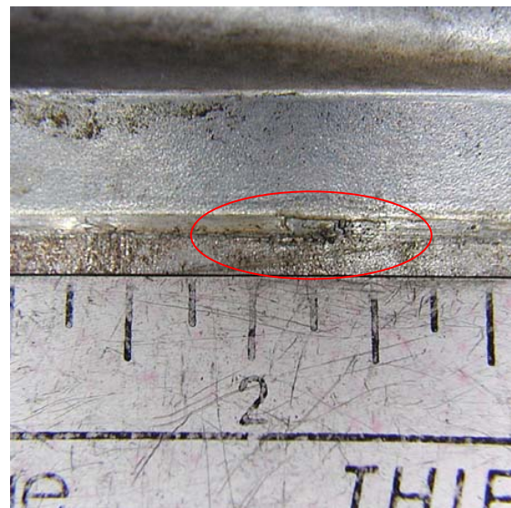
This close-up photograph shows where a crack was identified on unit 2. The crack was verified using UT in place and ET when removed. Best viewed at 200% zoom.
