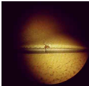
Platform crack in TBC coated bucket.
