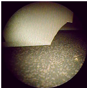
This is a stage 14-R tip failure
